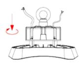
2. Tighten the screw. (This step can be omitted if there is no screw hole.)
