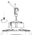
2. Tighten the screw. (This step can be omitted if there is no screw hole.)
